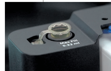
Onboard vortexing just prior to sampling ensures proper resuspension and delivers improved QC results and consistency.
