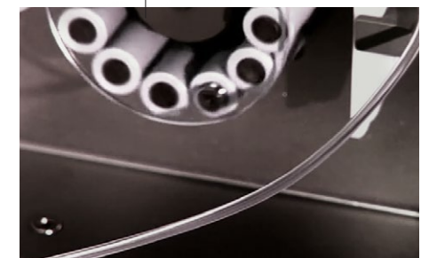
Samples are delivered to detectors in an air-gap delimited stream as part of a patented, rapid microvolume sampling process.
